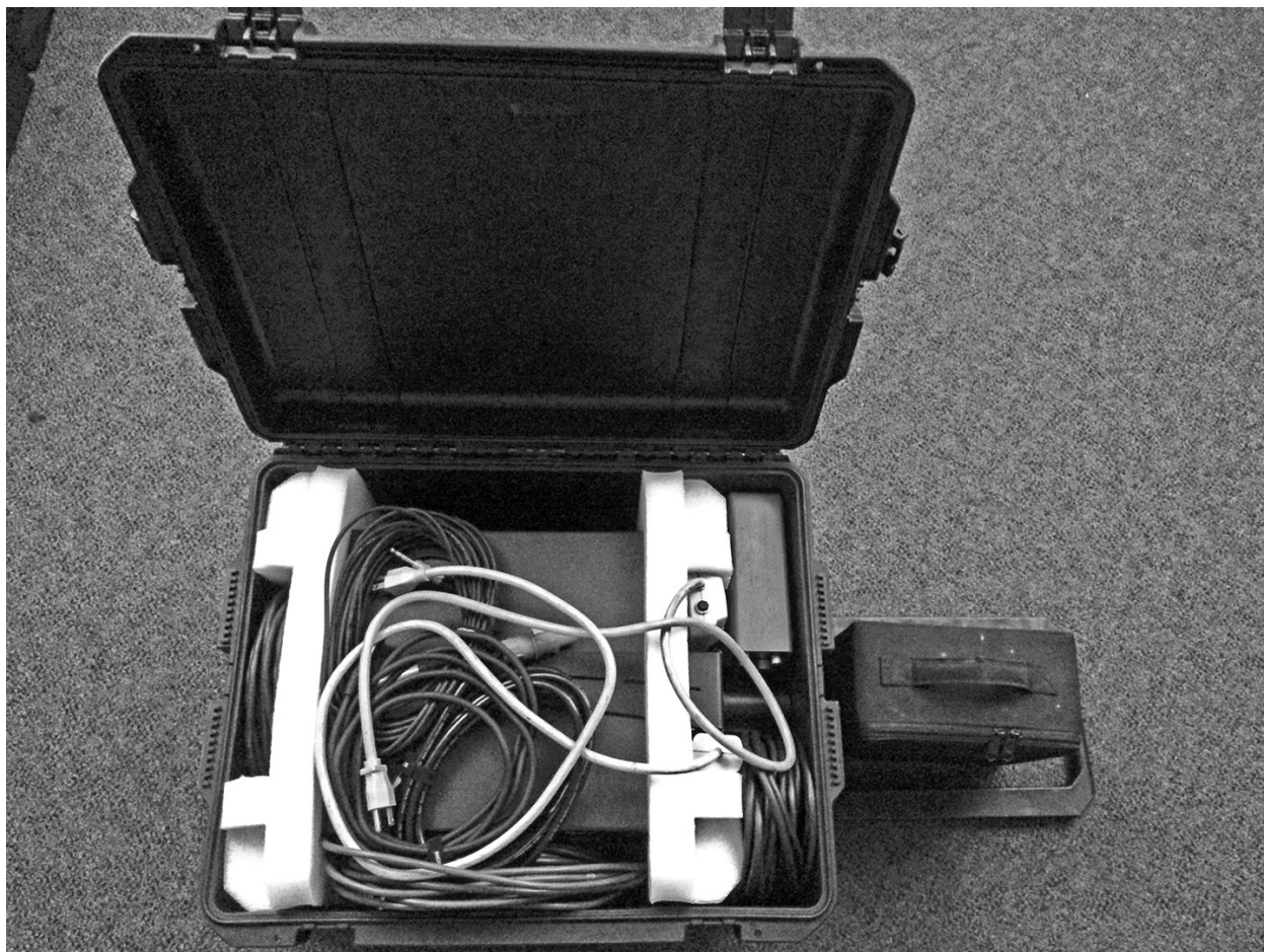
The PAIRS packed into the Pelican case, with Brahma microphone at left, ready for transport
