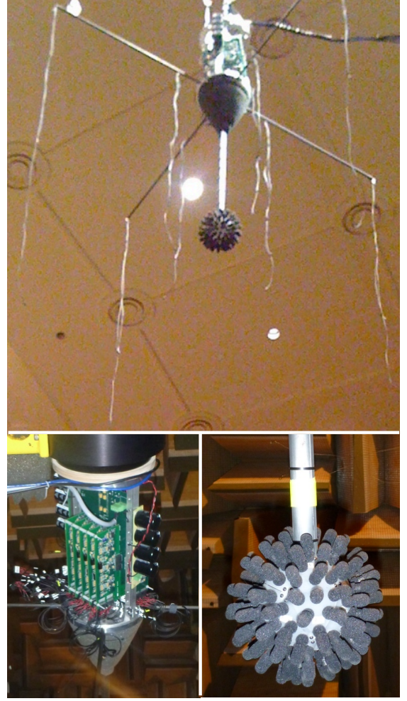
Figure 4: The SAM-array with outriggers (upper picture), and close-ups of the onboard electronics (left) and of the inner sphere (right).
